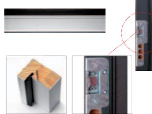
Wooden doorframe ENERGO 68 mm is made of glued pine wood, covered with an aluminium shape coated with a PVC coat in the colour of the door and threshold with a thermal inlet.
