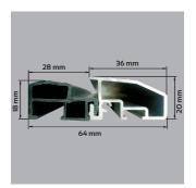
ALUMINIUM THRESHOLD WITH THERMAL INSERT
