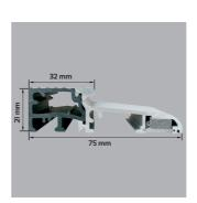
**ENERGO THRESHOLD** WITH THERMAL INSERT
